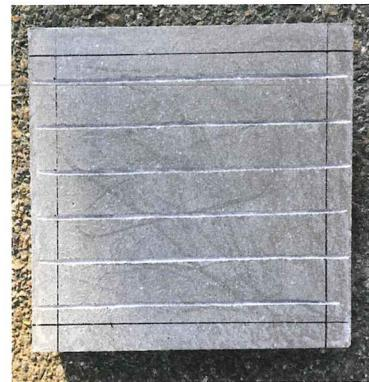
Fig. 5 Grooved concrete bed
