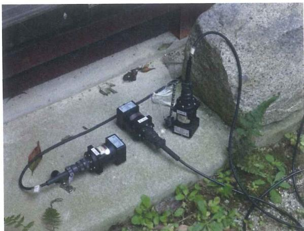
Photo. 10 Microtremor experiment of the ground
