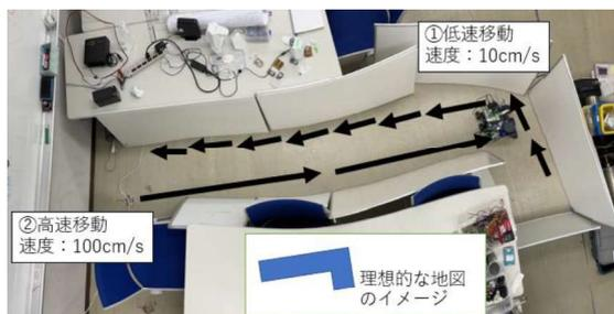
Fig.6 Diagram of the experiment overview
